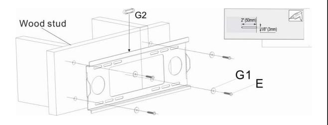
CAUTION: Do not over-tighten bolts-doing so many cause unnecessary damage to the wall. Avoid excessive torque.
